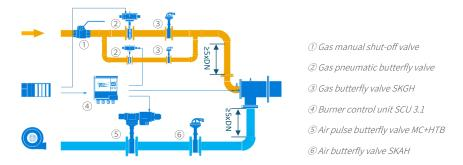
High/low pulse control. Two gas branch line: open one gas pneumatic valve for low capacity, two for high capacity.
